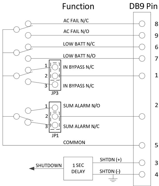
**Figure 8 : Simplified Schematic of Interface Connections**
