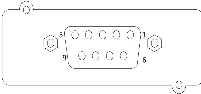
**Figure 9 : DB9 Output Connector Isolated Contacts Card**
