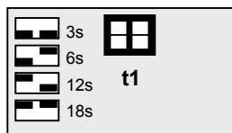
DIP switch pack **t1** determines the circuit breaker's response time to an overload condition. Response times of three seconds, six seconds, twelve seconds, and eighteen seconds may be selected as shown to the left. The t1 DIP switches are factory set for a response time of eighteen seconds. POWERVAR recommends that these settings not be changed without first consulting POWERVAR Technical Support.
