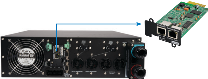
The bundled Network Card-MS allows the 9PX to connect to an Ethernet network and the Internet, supporting real-time monitoring and control of UPSs across the network via a standard web browser, SNMP-compliant network management system or power management software
