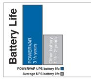
The design of the POWERVAR UPS utilizes automatic voltage regulation (AVR) technology, reducing the number of times the UPS switches to battery power. This design increases the life of the battery and will save you the cost of frequent battery replacements.
