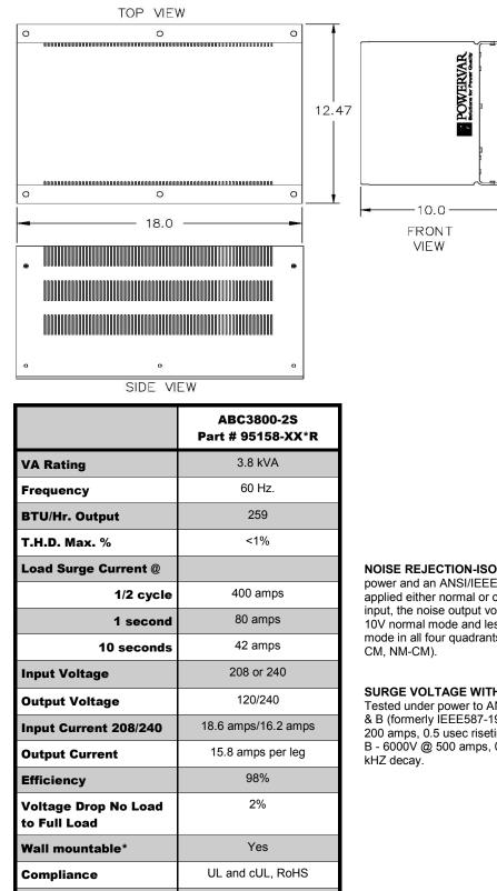
NOISE REJECTION-ISOLATION: With unit under power and an ANSI/IEEE C62.41Cat. A pulse applied either normal or common mode at the input, the noise output voltage will be less than 10V normal mode and less than 0.5V common mode in all four quadrants (CM-NM, NM-NM, CM-
