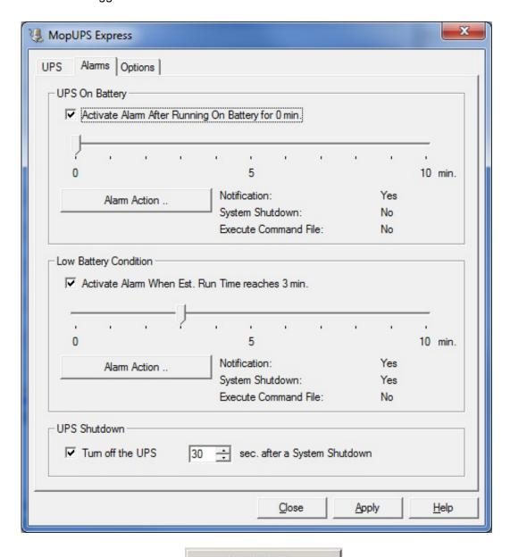
Press the Alarm Action button to configure what you want MopUPS Express to do when the condition is sensed and the delay has elapsed.
