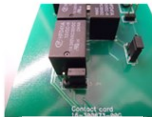
Figure B6 JP1 jumpered 2 to 3
